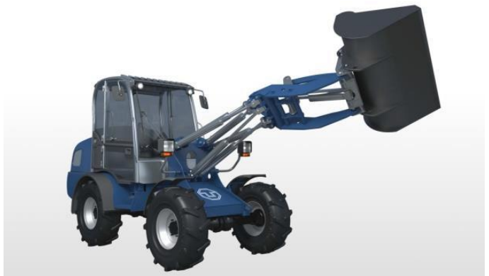
Figure 1: Hexapod wheel loader with the possibility of working movements in six degrees of freedom.
