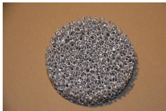
Figure 1 Metal Foam (10 ppi, stainless steel, Fraunhofer IFAM)
